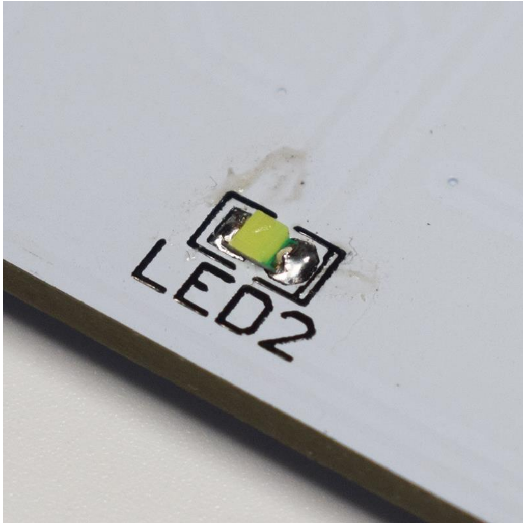
The green dot of this LED corresponds to the pad on the right.
